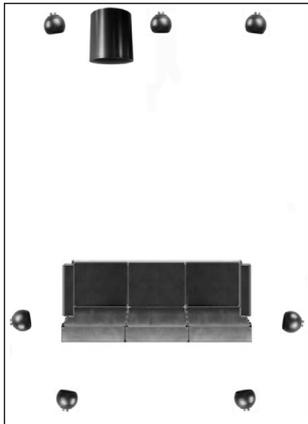
***Typical setup of a home theater system consisting of seven Micro SE speakers and a TR-1D subwoofer***
